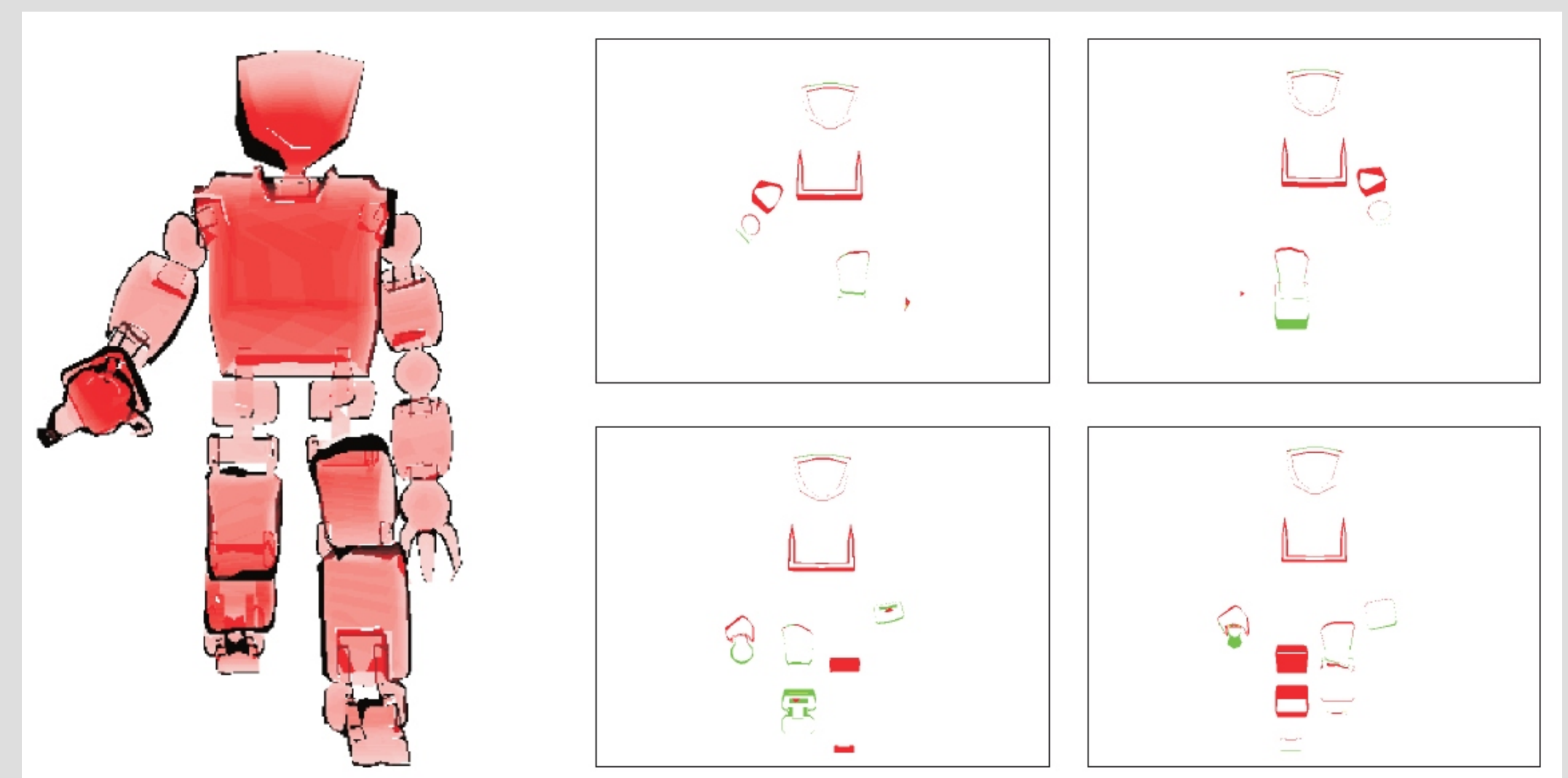
Due to the high voxelization performance, per-frame voxelization of an animated dataset is possible. In this example, the robot model is rendered with a walking animation from a constant viewpoint. Voxelization slices for four example frames from the animation are shown in the panels on the right hand side (all panels show the same slice index).
