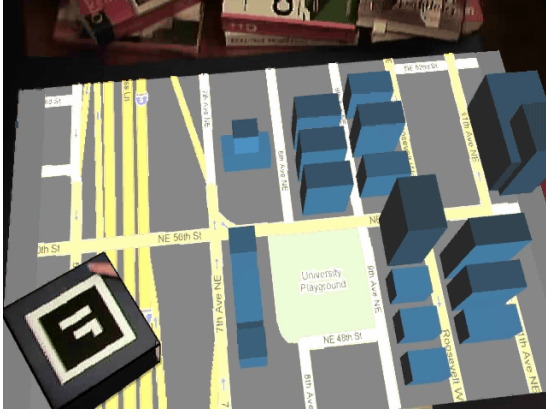
Figure 3: Tangible interaction zone with superimposed graphical augmentations. This image shows the same view as Fig. 2. Note that the base plate is rendered as a textured quadrangle depicting a street map. (In this rendering, the phantom model used for the physical prop is represented as an overlaid black wireframe mesh.)
