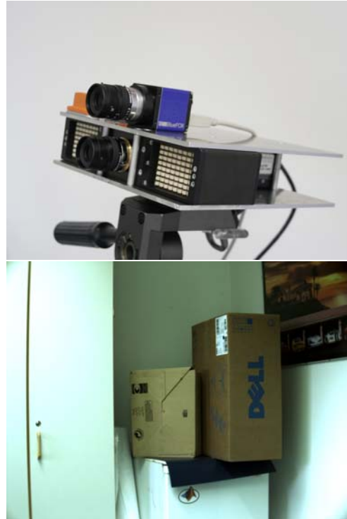
Figure 2: Our two-camera setup (top). The high resolution color camera is attached to the top of the time-of-flight PMD camera. The bottom image shows the color image delivered by the color camera for the example scene.
