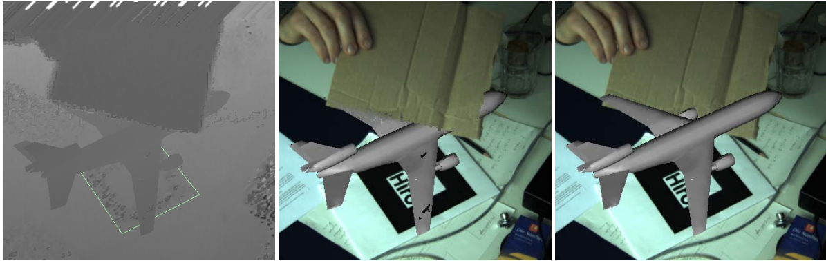
Figure 7: Virtual DC10 plane model occluded by real piece of cardboard. (Left: depth data. Center: AR image with occlusion handling. Right: conventional AR display without occlusion handling.)
