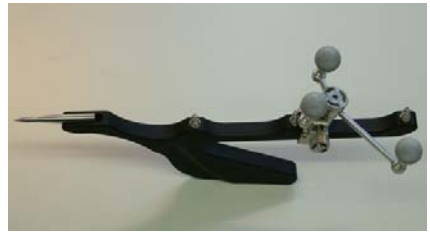
Figure 3: Example of a tracked tool used for interaction.
