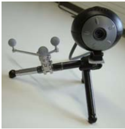
Figure 2: Webcam with attached marker clamp.
