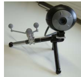
Figure 2: Webcam with attached infrared marker spheres
